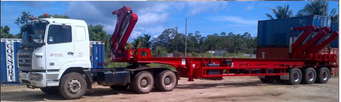
The new 3 crane side lifter which will assist KPS in moving its clients containers
